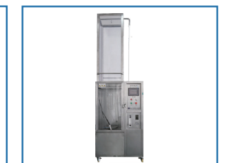
IPX5&X6 rain test chamber
